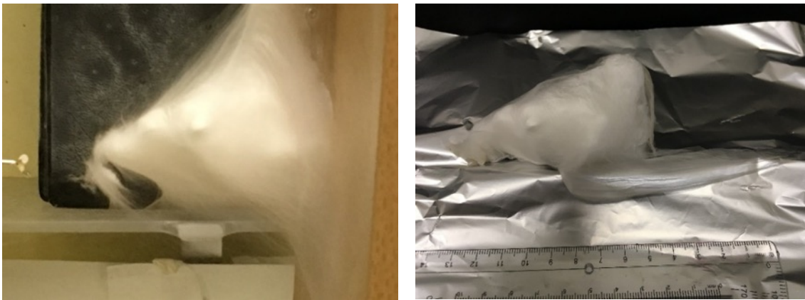
Figure 4.19 Macroscopic view during and after electrospinning of \text{CaCl}_2 3w/w% solution. [24]
