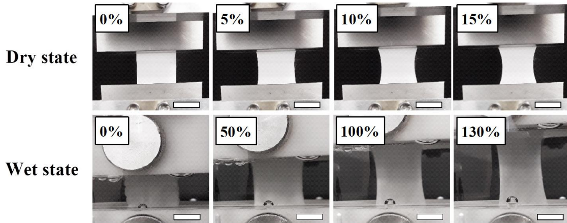
Figure 20 Representative macroscopical images of mechanical tensile test of PSI in a dry state and PASPDAB in a wet state at different elongations. Scale bars indicate 1 cm. The figure was adapted from [RP2] [131].
