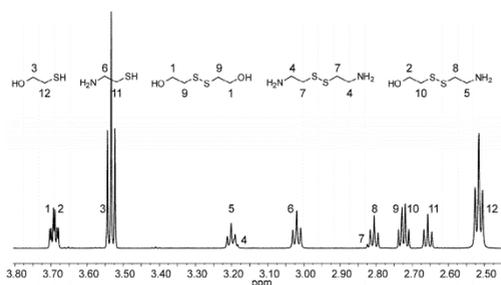
**Figure 2.** <sup>1</sup>H NMR spectrum of the 12 different methylene peaks of the five different compounds (from left to right: MSH,
