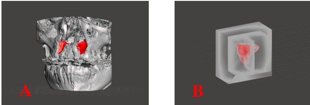
9. Figure Meshmixer program completes the final shape of the graft (A), while CAD program is used to plan the mold of the graft (B).
