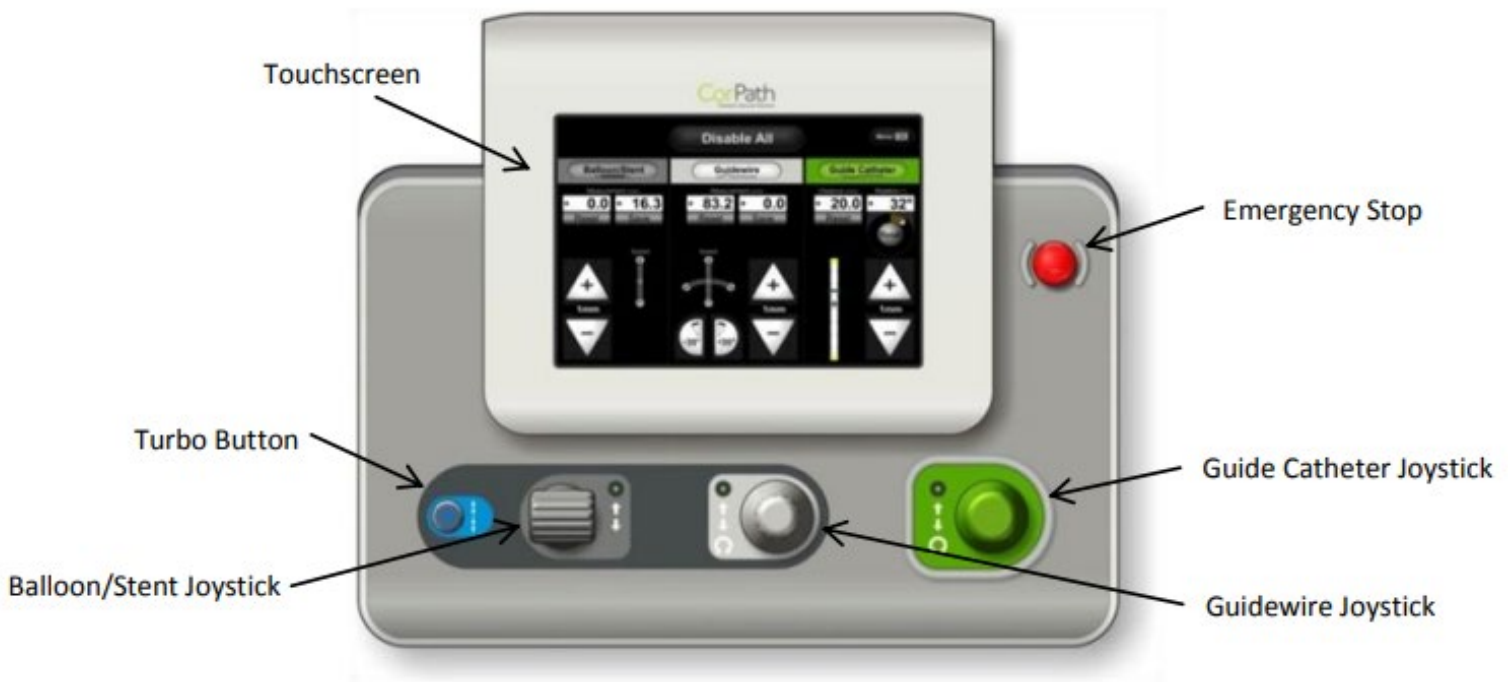
Figure 5. CorPath GRX Workstation for robotic control. The touchscreen displays the device coordinates and allows stepwise precision control of the endovascular tools. Three joysticks serve for guide catheter, guidewire navigation, and balloon/stent positioning. The turbo button accelerates device exchanges. (27)
