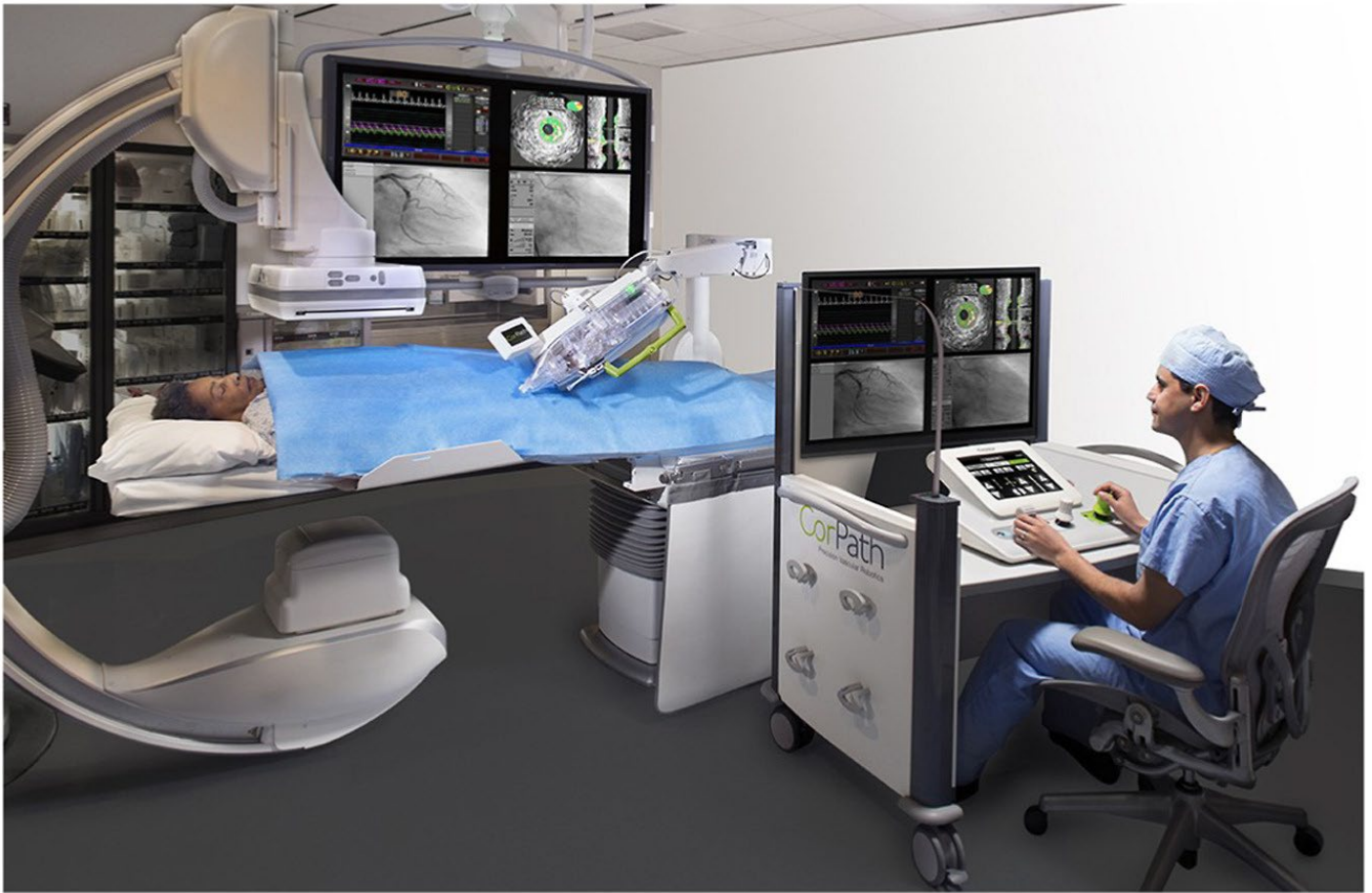
Figure 2. A schematic figure to demonstrate the parts and setup of the CorPath robotic system. The interventional cockpit is radiation shielded. The operator sits throughout the robotic interventional part and coordinates the robot with the control console. The bedside component is attached to the operating table. Endovascular devices are loaded in the robotic system.(26)
