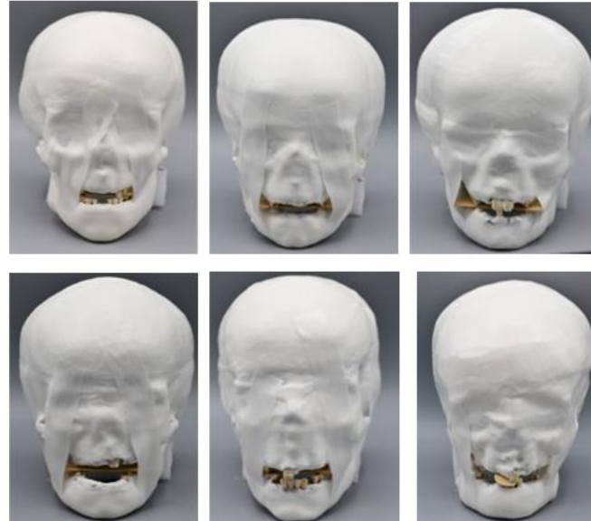
Figure 7. - Dimicleft series: age-specific anthropomorphic radiological phantoms with artificial orofacial clefts
