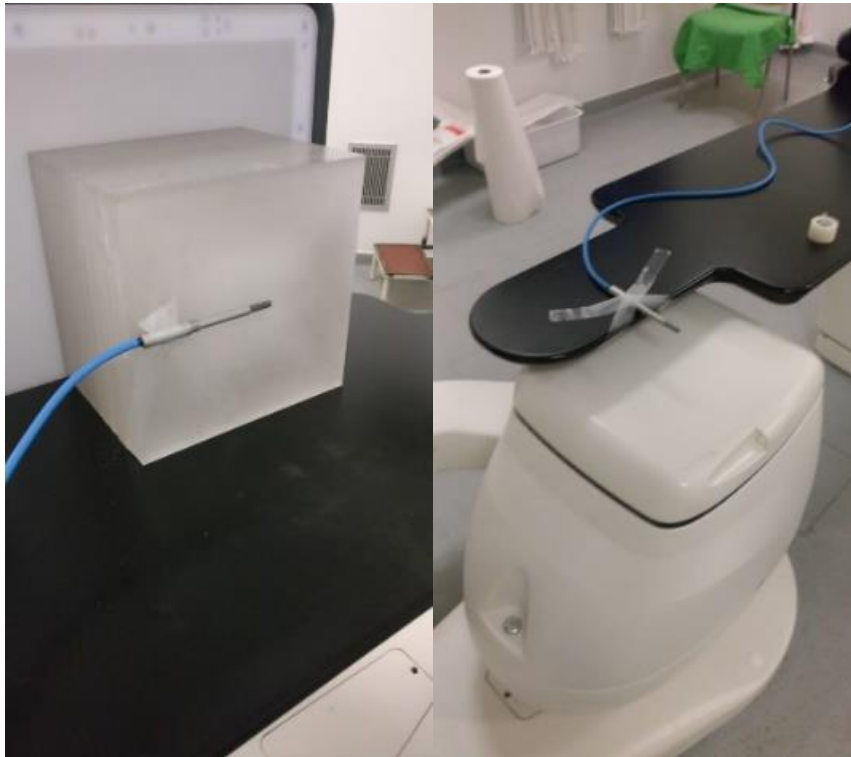
Fig. 3. Geometrical set-up for the measurement of ESAK (left, includes backscatter) and IAK (right, without backscatter) which were used to determine the accuracy of displayed dose indices.
