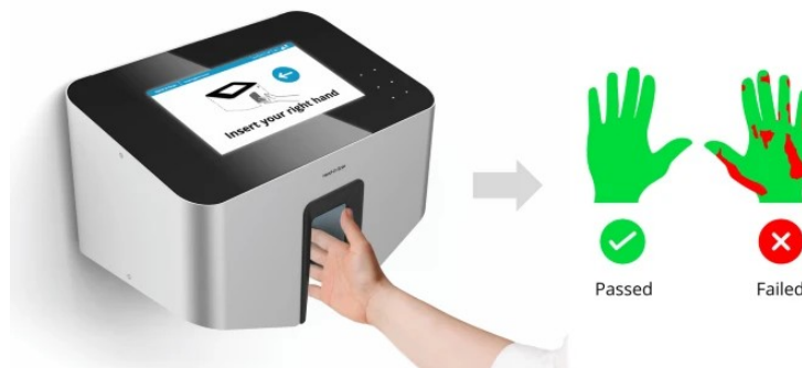
Figure 1. Hand coverage was measured by the Semmelweis System, which automatically analyzes coverage and provides visual feedback: on the user interface provided outcome green indicates handrub-covered areas, while red indicates areas not covered by handrub [2, 33].
