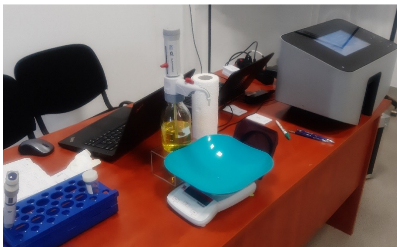
Figure 3. Experimental setup for quantifying handrub spillage [49].
